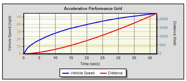
Acceleration Performance: TIME TO ACCELERATE ON A 0.00% GRADE TO 55.0 (MPH) IS 42.20 (SECS)
